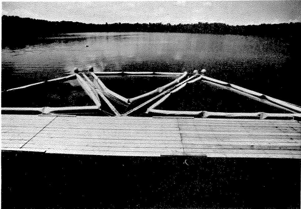
Figure 4. Top edge of 3 triangular limnocorrals suspended in the Bay of Quinte.
